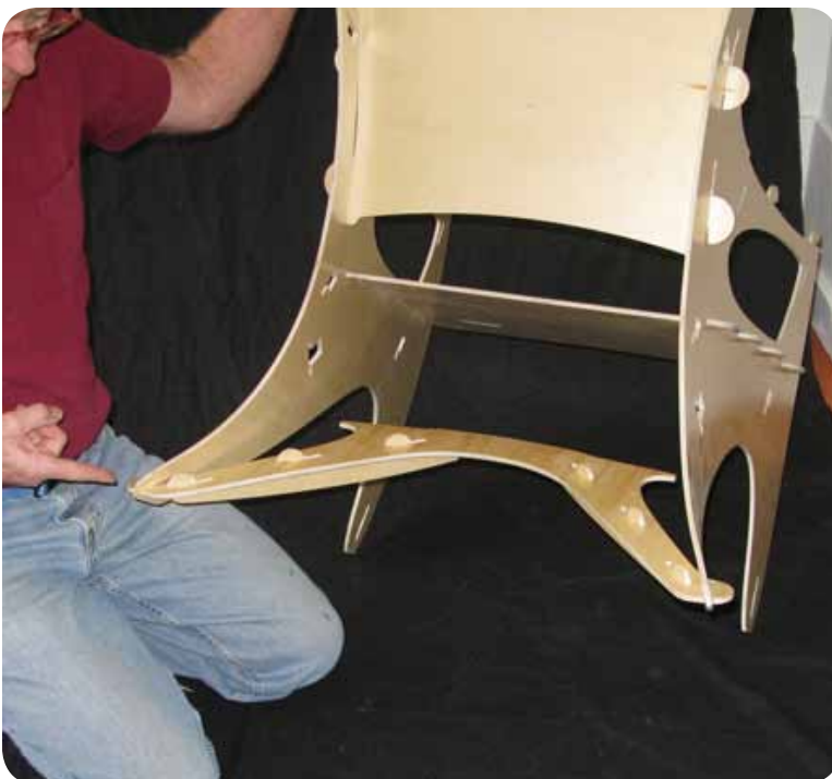
Pic 12 bend the other side's leg away so it will engage too. Caution: parts under tension at this point, they could recoil and hurt you.
