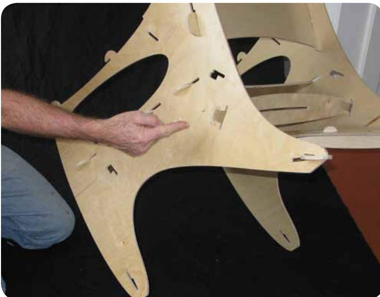
Pic 13 one end of stretcher bar locked into one side.
